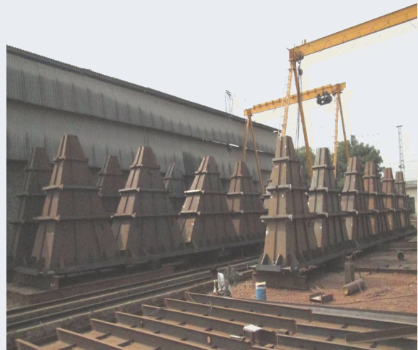
Bunker hoppers assembly
