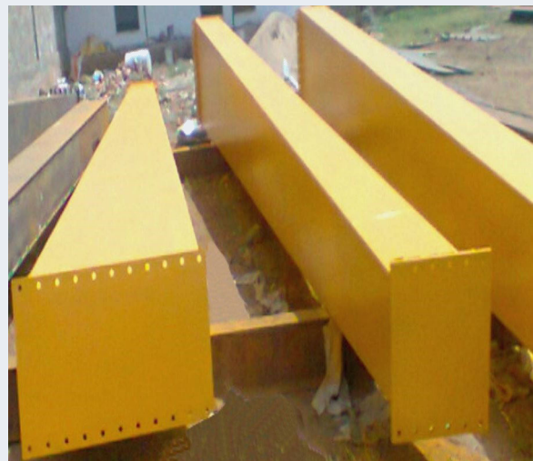
60 MT crane vertical supports
