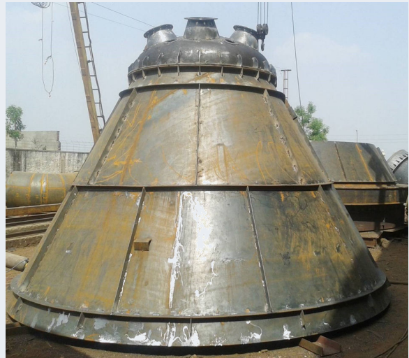
Fly ash & Bed ash silo assembly
