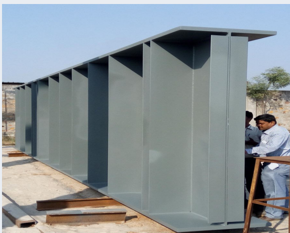
Girder for Project : RSPL Limited Height : 2.6 m , Weight : 18.0 MT
