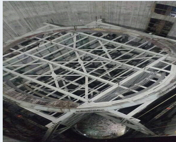
Base Frame for Boiler Module for Project : Dangote Oil Refinery Limited Size : 13.0 m x 45.0 m , Weight : 140.0 MT
