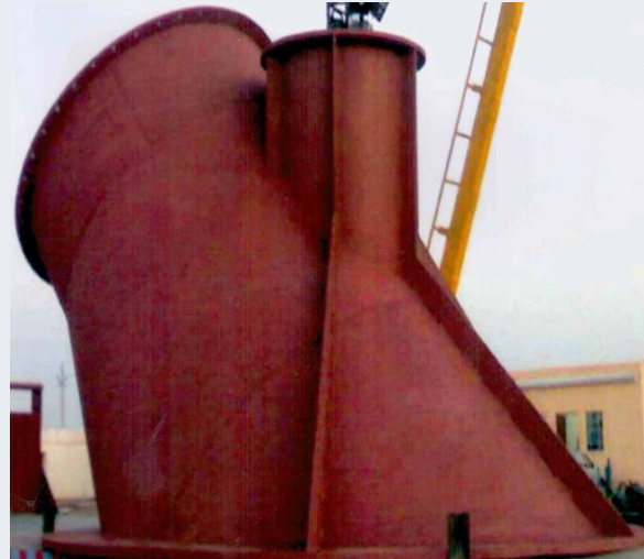
Separator outlet duct
