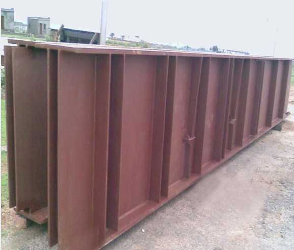
Built-up Beam Height - 1.36 m, Weight - 8.0 MT
